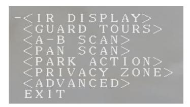
IR DISPLAY – Allows you to view advanced parameters on the status of the IR illuminator real time
